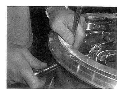
Place the washer on the backside of your rim. Install the Nylock Nut onto the stern. Use the supplied standard jam nut on the external threads-temporally- to allow you to tighten the Nylock securely, but not so much that the grommet squeezes out
