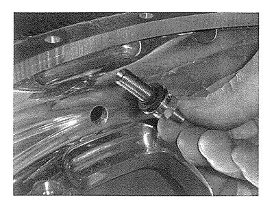
Select the correct grommet for the hole. Insert the stem through the grommet and then through your rim.
